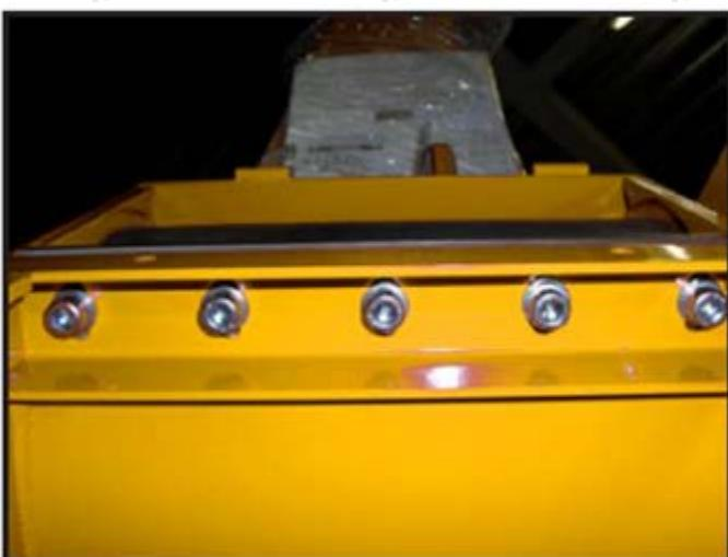
The shredder is a machine for shredding/chipping newly cut wood. The rotor has 2 blades each with a 30 cm width and is powered by a gasoline engine. Transmission is through two parallel drive belts. The shredded wood or chips are discharged through the output tube by the centrifugal force of the rotor. Because of the angle of the blades, branches are pulled inside the machine automatically and no feeder belt is required.
