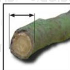
You should not use the shredder for shredding/chipping metals, stones and plastics. If you are going to shred tree roots, check if the diameter is less than 10 cm and remove all earth, sand and stones.
