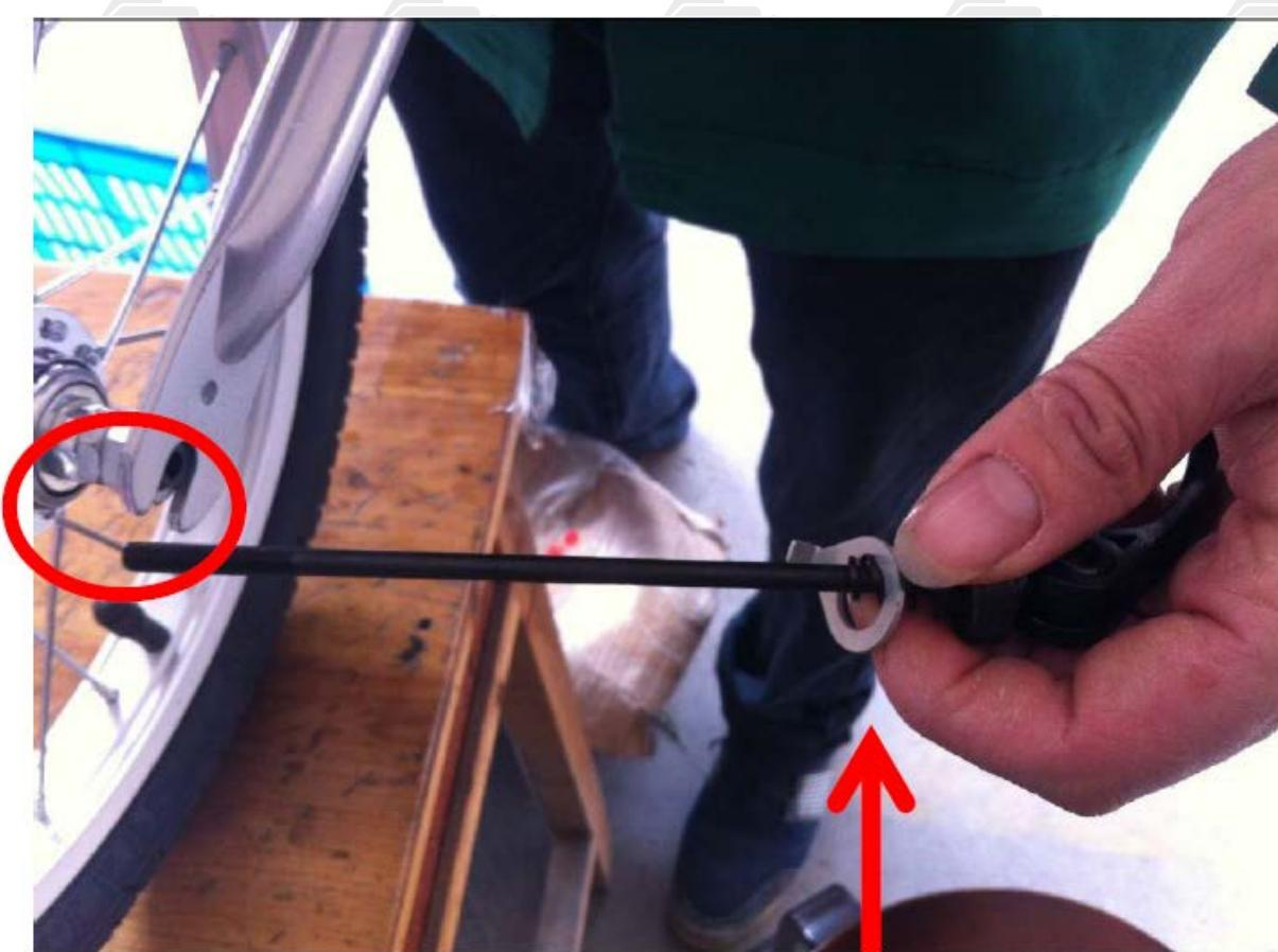
Fit wheel onto forks, with outer axle sitting flush with fork inset. Ensure that one side of the fork lock clamp and the washers are on inner axle rod.
