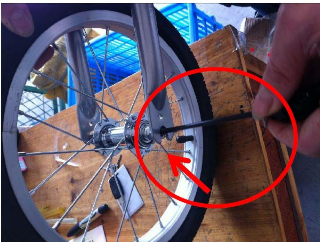
Insert inner axle shaft. Shaft will slide through the outer axle shaft from one side to the other and extend past fork.
