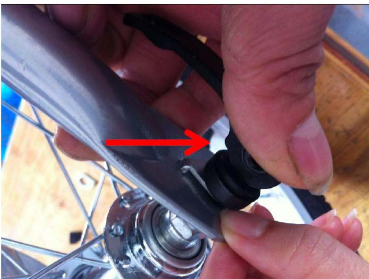
Tighten the inner axle shaft clamp and then lock it down to ensure a tight fit.
