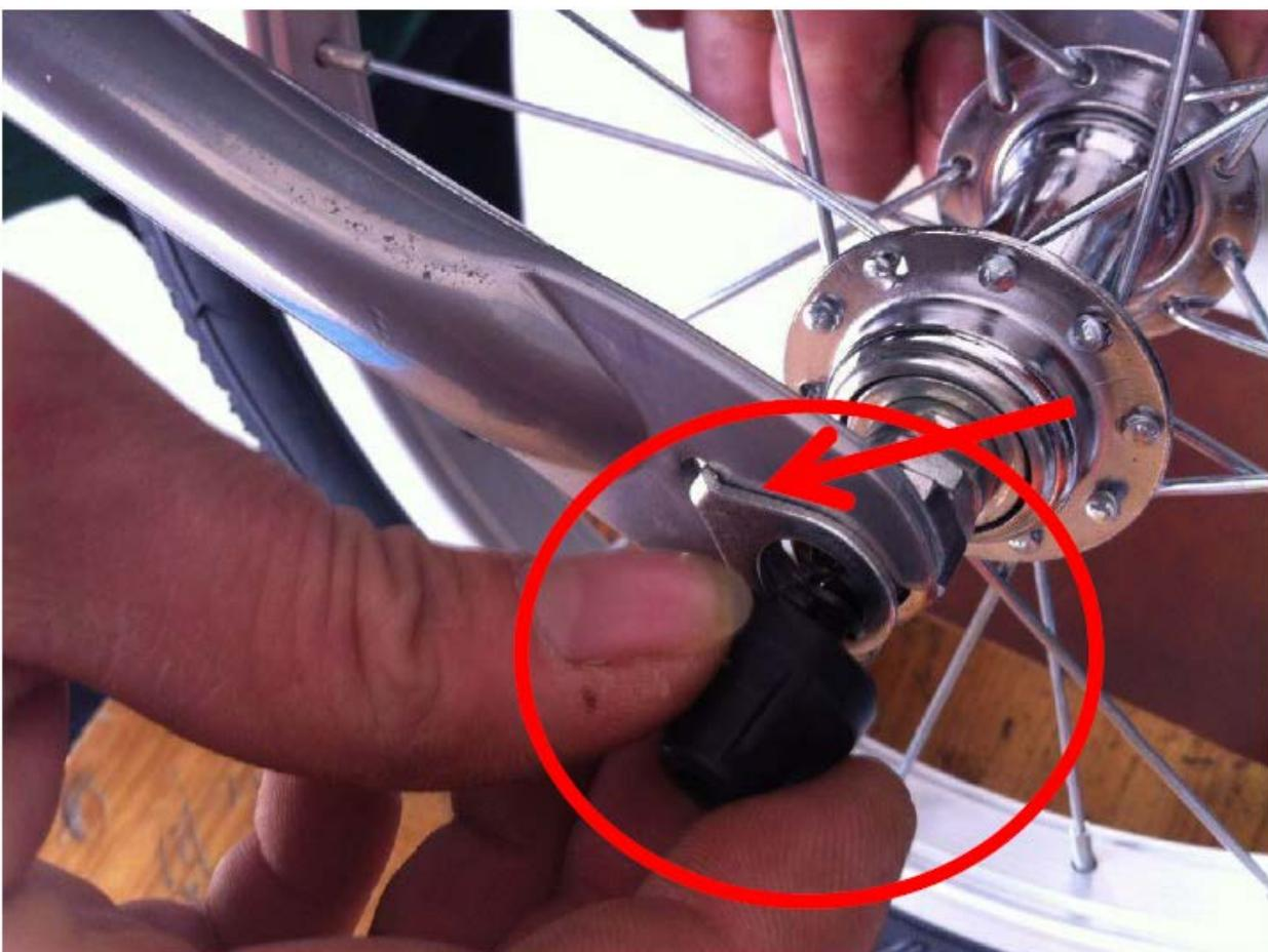
Fit the fork lock clamp and washers and then attach the inner axle rod nut.
