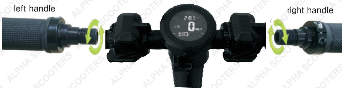
1. Insert the left handle into the socket and rotate it in an anti-clockwise direction until it's tight and secure.
