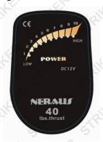
There are 10 LED on the meter, 7 upper LEDs are green and 3 lower LEDs are red, when all the green LEDs are turned off, that means the input voltage is lower than 10.25V, you must turn off the motor and disconnect the motor from the battery, otherwise it may cause forever damage to the battery.
