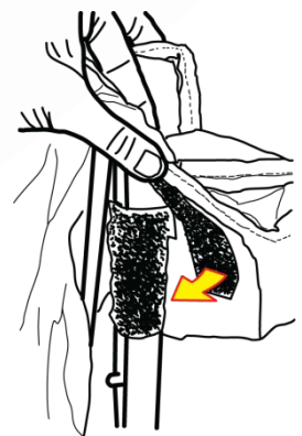
Figure 2 – Canopy to Leg Velcro Attachment
