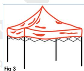
3. With the corner of the roof over the corner of the frame, carefully fully extend the corners by pushing in the lock pin and pushing up the frame (*the roof may need to be folded half way up so the roof is clear and does not get caught and possibly damaged*).
