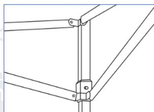
4. Once frame is fully extended, straighten up roof and velcro corners.
