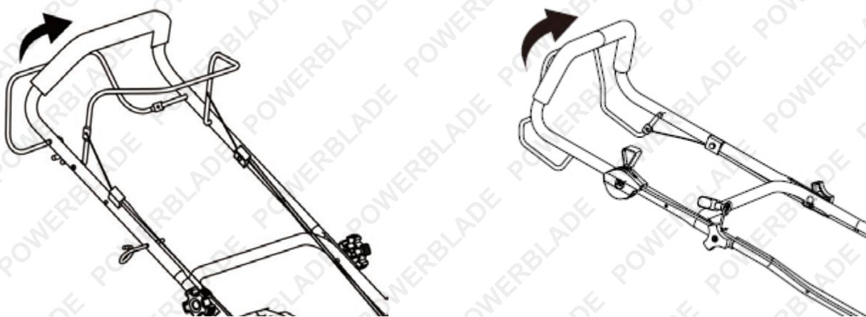
This unit equipped with a self-propelled system. If you press the drive lever (clutch lever), the clutch for the drive will be closed and the lawnmower will start to move with the engine running.
