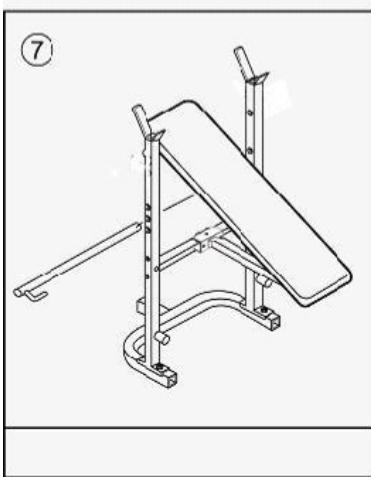
Insert the bar into the holes in the Upright Frames.
