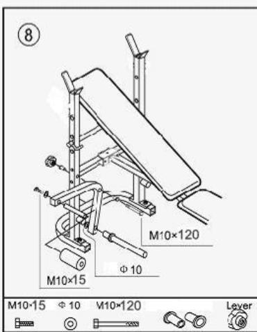
Assemble the two fly arms(9) first,bolts the Round tubes(11) (10) to the arms(8,9) with The M10x20 bolts. Push the form pads Onto the form tubes(10). Attach the fly Arms to the upright post with M10x130mm Bolts,metal bushes(17) and levers(16)
