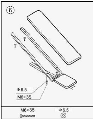
Slide the Backrest Frames onto the pivot Bar on the Cross Bar,then screw the Backrest to frames.
