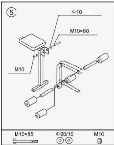
Bolt the leg Extension Bracket to the Front Leg using the Thicker Bolt and two Washers.Slide the Round Tubes into the hole provided.Push the Foam Pads onto the tube.
