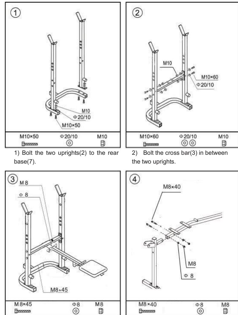
Bolt the main beam(6) to the center of the cross bar(3).insert the pull pin to hole of the cross bar.
