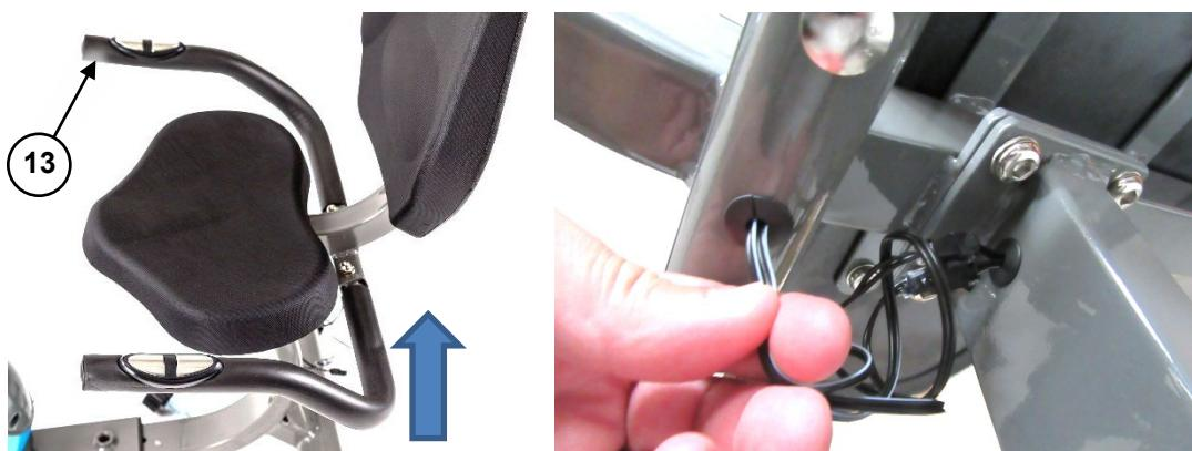
8. Pull the cable connection bracket (D) and wiring from the main body tube (where the front mounting tube is to attach). Ensure that the cable connection bracket and wiring remains in position by itself and does not slip back inside the tube. Then, carefully slide the front mounting tube (14) over the main body tube – ensure that the front mounting tube slot (E) is facing toward the seat and tensioner and wires remain in position and do not get caught or pinched between the tubes.
