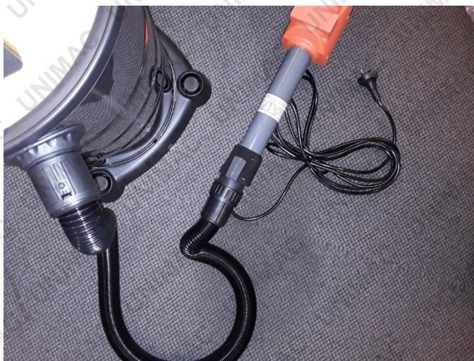
Plug drywall sanders' power cable into supplied power point on vacuum.
