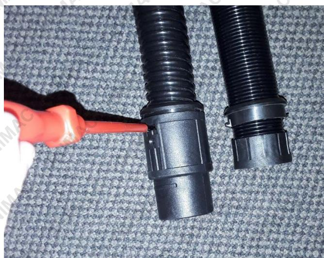
3. Connect adapter from the vacuum to the opposite end of the drywall sanders' hose. Line up the windows from the adapter with the clips from the hose and apply pressure with the 2 pieces together to lock them into place.
