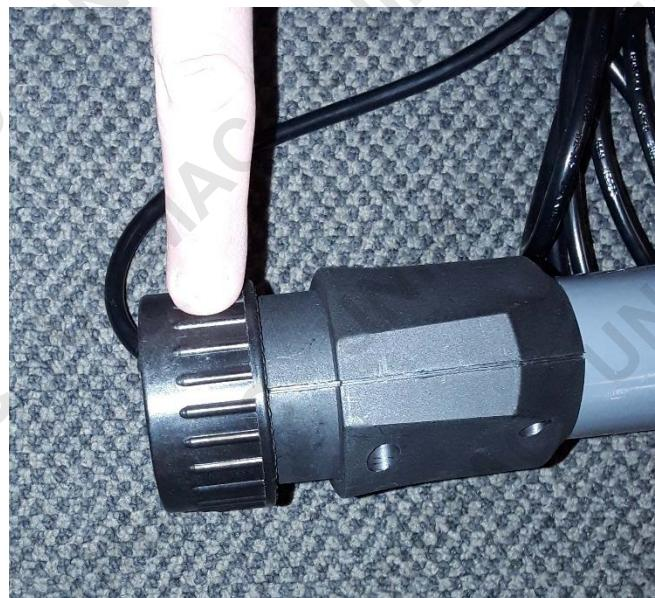
2. The unit comes with 2 adapters, use the smaller of the 2 . Line up the windows on the adapter with the clips from the hose and apply pressure with the 2 pieces together to lock them into place.
