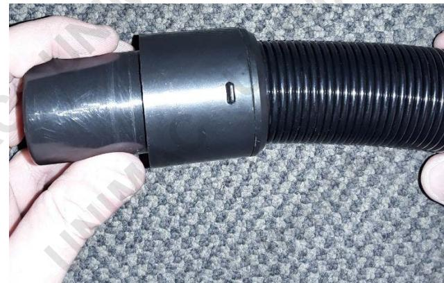
3. Once the adapter is connected to the hose, insert the adapter into the drywall sander and tighten the large locking nut to ensure the hose doesn't come loose.
