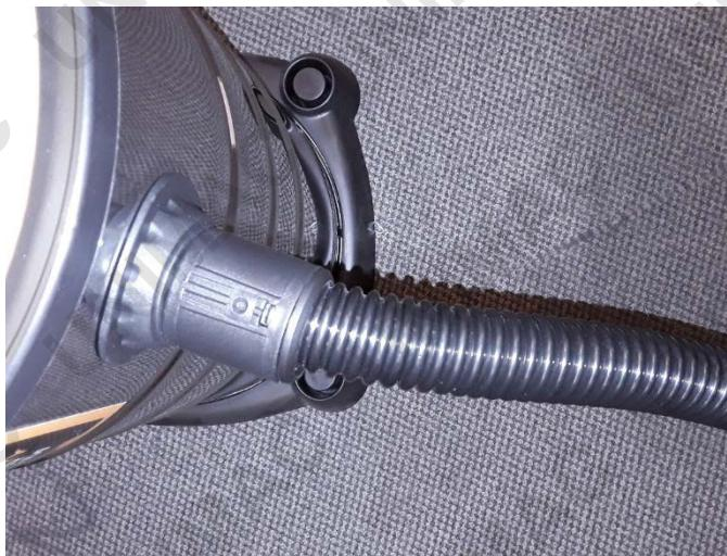
2. Remove the adapter connected to the vacuums hose.
