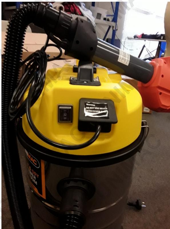
Once ready, use switch 2 on vacuum. The vacuum will auto-engage and disengage after a few seconds when the drywall sander is in the corresponding on or off position.
