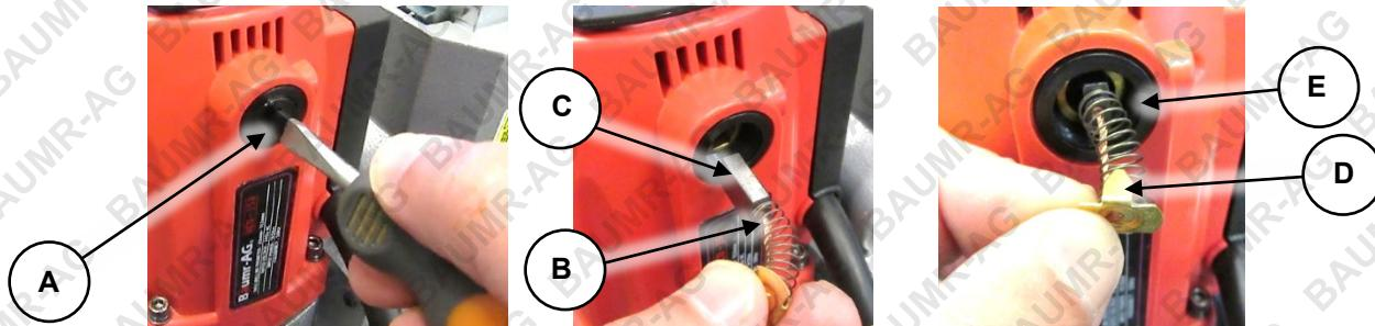
3. Insert the brush into the cavity – the brush has 2 prongs on the electrical conductor (**D**) – ensure these sit in the slots (**E**).
