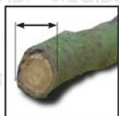
You should not use the shredder for shredding/chipping metals, stones and plastics. If you are going to shred tree roots, check if the diameter is less than 10 cm and remove all earth, sand and stones.
