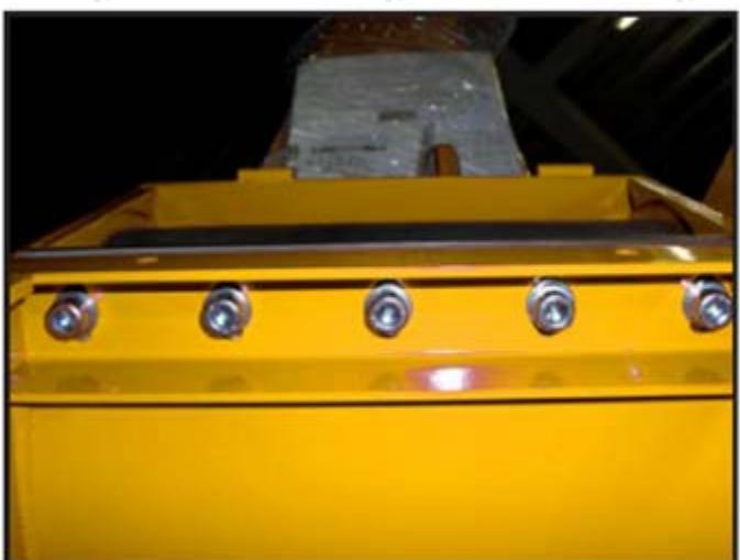
The shredder is a machine for shredding/chipping newly cut wood. The rotor has 2 blades each with a 30 cm width and is powered by a gasoline engine. Transmission is through two parallel drive belts. The shredded wood or chips are discharged through the output tube by the centrifugal force of the rotor. Because of the angle of the blades, branches are pulled inside the machine automatically and no feeder belt is required.
