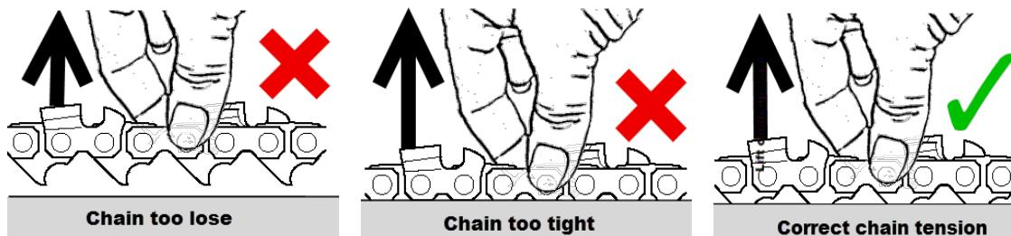
10. If chain is too loose or too tight, loosen the nuts **before** adjusting the chain tensioner. Failure to loosen the nuts will strip the tensioner and void your warranty.
