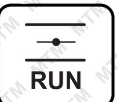
When the engine is warm, place choke in RUN or OPEN position.
