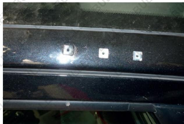
9. Install snorkel body to vehicle using three nyloc nuts and body washers provided and attach to pillar bracket using M6 bolts and washers provided.
