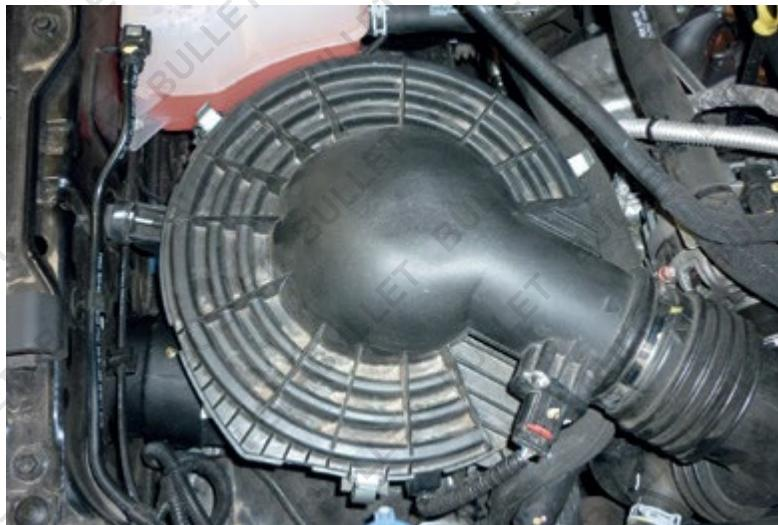
18. Pull wiring for side marker indicator through snorkel body and attach indicator to snorkel.
