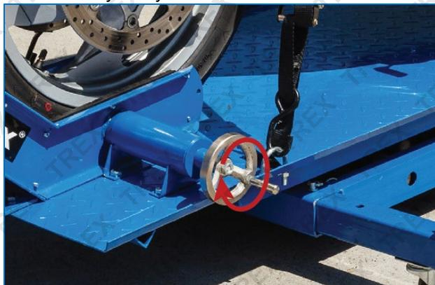
4. Tie down and anchor motorcycle handles with rope and anchor points
