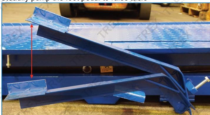
6. Once work has been finished on motor cycle, gently press down smaller pedal with a constant pressure until table is fully lowered
