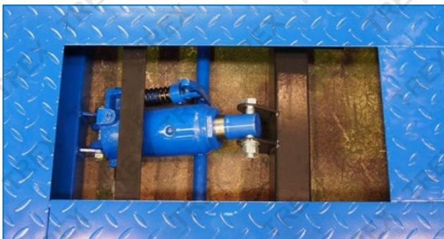
2. Remove hydraulic cap from pump and fill with hydraulic jack oil (or ISO 32 hydraulic oil)
